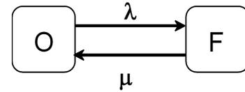
Fig. 1. Two-state model of electric system component
