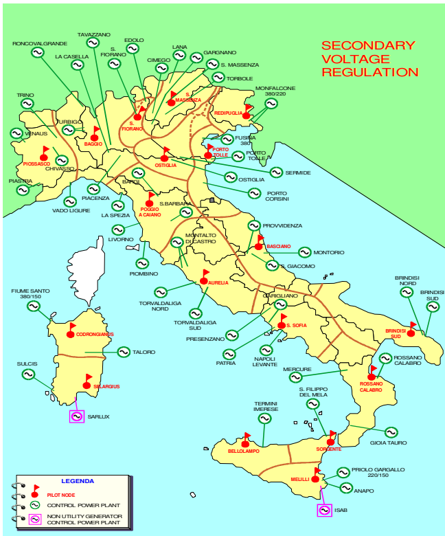
Fig. 2. Application plan of the Italian hierarchical voltage control system
