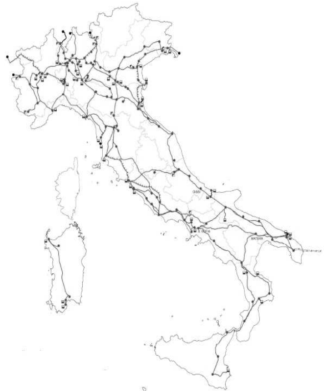
Fig. 3. 380 kV-50 Hz Italian transmission grid.
