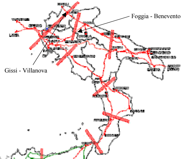
Fig. 2. Critical grid sections in Southern Italy [1]
