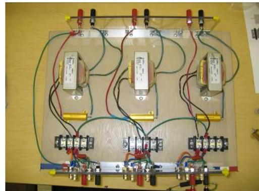
Fig. 10. Actual layout of the three-phase auxiliary voltage source of Fig. 9.
