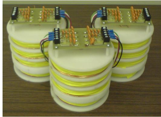
Fig. 6. Transmission line prototype for a 2-mile section.
