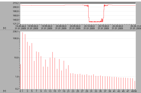
Fig. 14. Fourier analysis of voltage at the ZDM 2500-DIMM Light output when the reduction of the lighting level is 67%.
