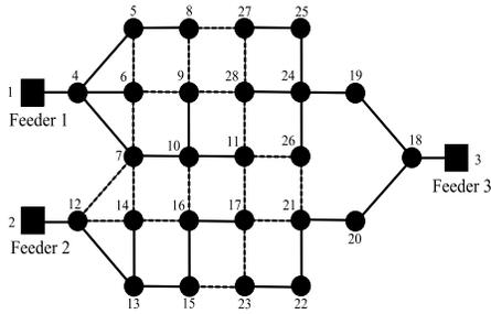
Fig. 2. DS with three feeders. It corresponds to a graph with three trees.
