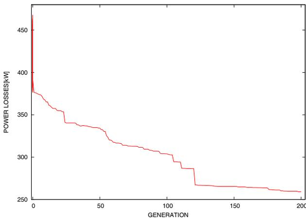
Fig. 7. Power losses in kW of the best individual in each population by generation.
