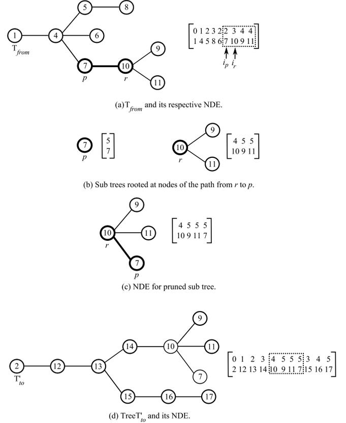
Fig. 5. Determination of  $T_{tmp}$  to the operator 2. In (a), the highlighted lines are the nodes in the chain from  $r$  to  $p$ . The depths in (b) and (c) are relative to choice of node 14 as adjacent node.
