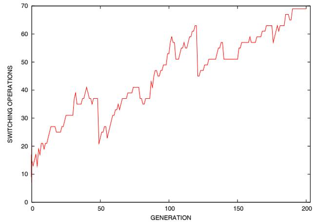
Fig. 8. Switching operations of the best individual by generation.
