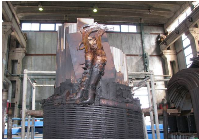
Fig. 5. Coil with demotion insulated paper
