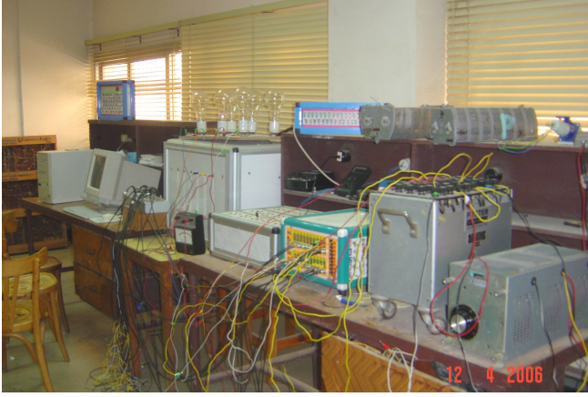
a. Experimental DSP-based setup of the laboratory transformer.
