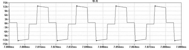
Fig. 12. Current in primary winding of transformer.
