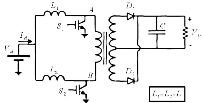
Fig. 2. Scheme of Dual Inductor Push-Pull Converter.
