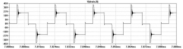
Fig. 11. Voltage on the primary winding of transformer.
