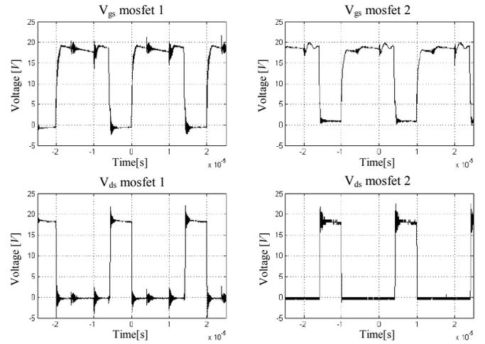
Fig. 21.  $V_{GS}$  and  $V_{DS}$  mosfet voltage.
