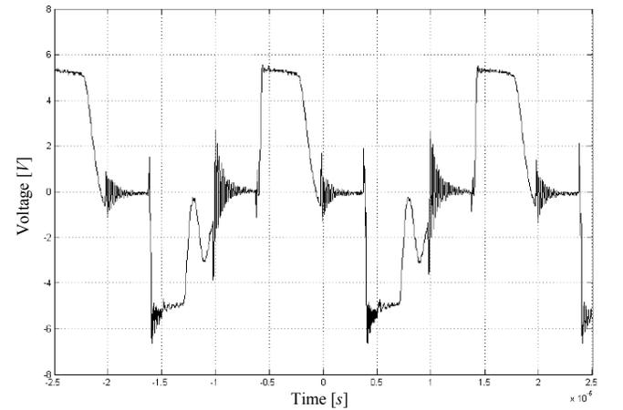
Fig. 22. Voltage on the primary of the transformer.
