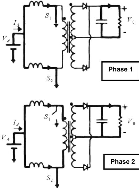
Fig. 3. Operation phases of the converter in CCM.
