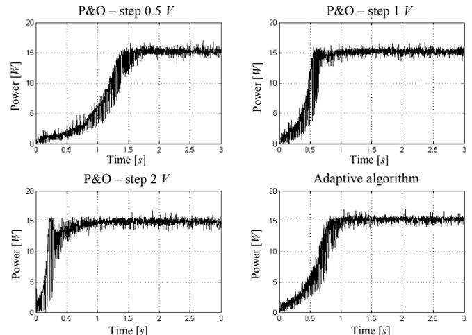
Fig. 16. Power in P&O and Adaptive algorithm.
