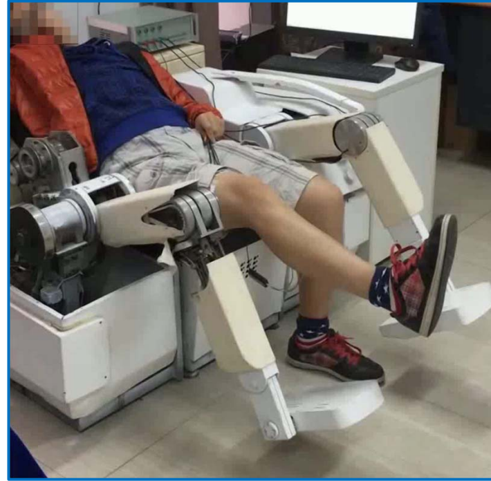
Demonstration of Robot Motion Control by sEMG
