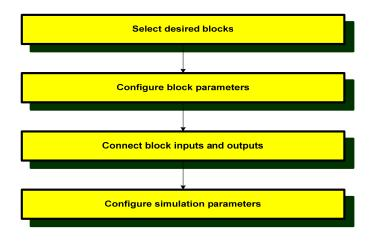
First you will gather all the necessary blocks from the Library Browser. Then you will modify the blocks so that they correspond to the blocks of the desired model. Lastly, but not the least, you will connect the blocks with lines to form the complete system and set the overall simulation parameters. After this, you will simulate the complete system to verify that it works.
