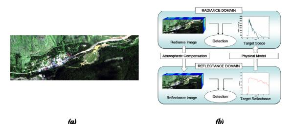
(a) True Color representation of the hyperspectral image analyzed; (b) Comparison of target detection schemes...
