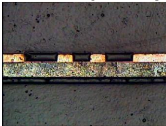
Diagram 2.3 – Cross section of product using flat-top copper plating.
