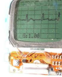
Wearable ECG monitor, for logging and analysis
