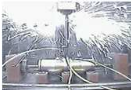
Fresh Sample, 100% Fails IIISC Test (N=3)
