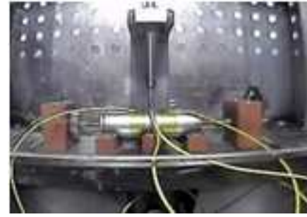
100 Cycle Aged Sample, 1 cell pass and 1 cell fail
