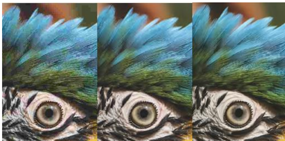
Fig. 2: Coded images of JPEG(left), JPEG2000(middle) and VVC(right) at the same compression rate (1/100)
