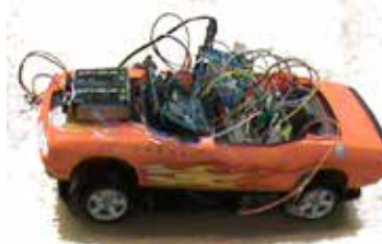
This Arduino-equipped toy car, built by Montgomery College engineering student Natnael Zewdie, has an IP address and can be controlled wirelessly from anywhere in the world.
