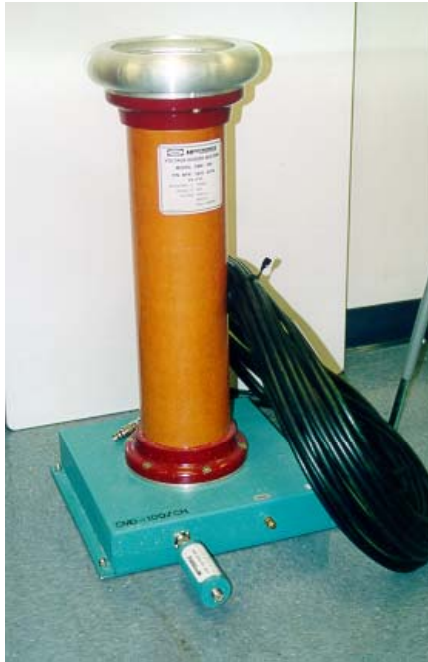
100 kV High Voltage Divider
