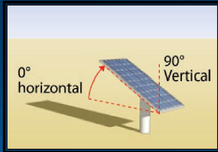
A tilt of 0 corresponds to a horizontal array, while a tilt of 90 corresponds to a vertical array.
