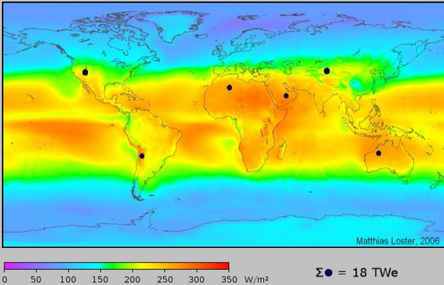
At 8% conversion, PV arrays at these locations would provide 18TW of energy.
