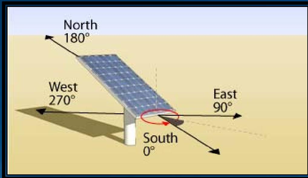
An azimuth of 0 corresponds to a south-facing array; 90 to an east-facing array; 180 to a north-facing array; and 270 to a west-facing array. Therefore, the azimuth of an array facing 20 east of south will be 20, while the azimuth of a PV array facing 20 west of south will be 340.
