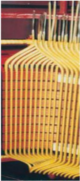
Each Coil Winding Has Multiple Turns
