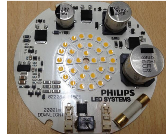
Example of “Driver on Board” LED module
