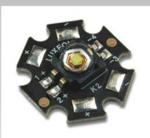
LED PACKAGE —An assembly of one or more LED die that contains wire bond connections, possibly with an optical element and thermal, mechanical, and electrical interfaces.
