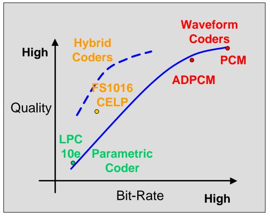
Hybrid Codecs employ tools such as vector quantization to gain quality at low bit rates.
