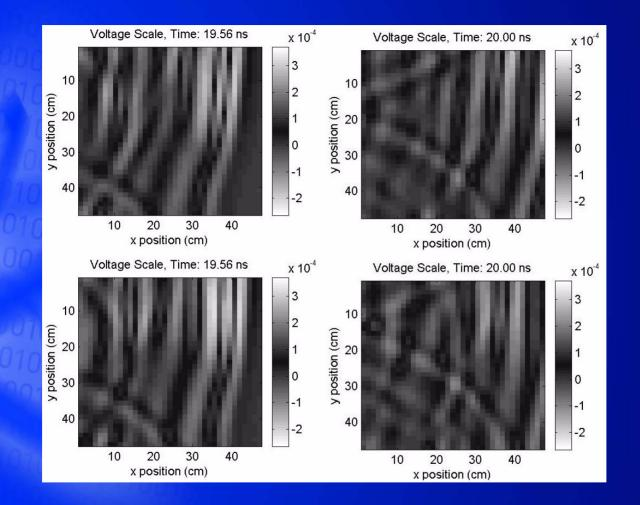
STA is LOS to AP at 3 m, separated by one soft partition
