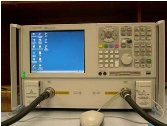
Agilent E8361A Network Analyzer 10 MHz to 67 GHz, 1.85mm test ports various coaxial and waveguide cal kits
