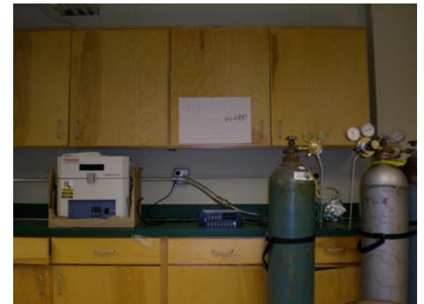
Chemical Vapor Deposition System For Carbon Nanotube Growth
