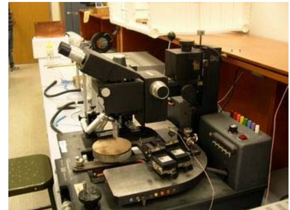
Probe Station with various probe Positioners DC to millimeter probes and calibration substrates
