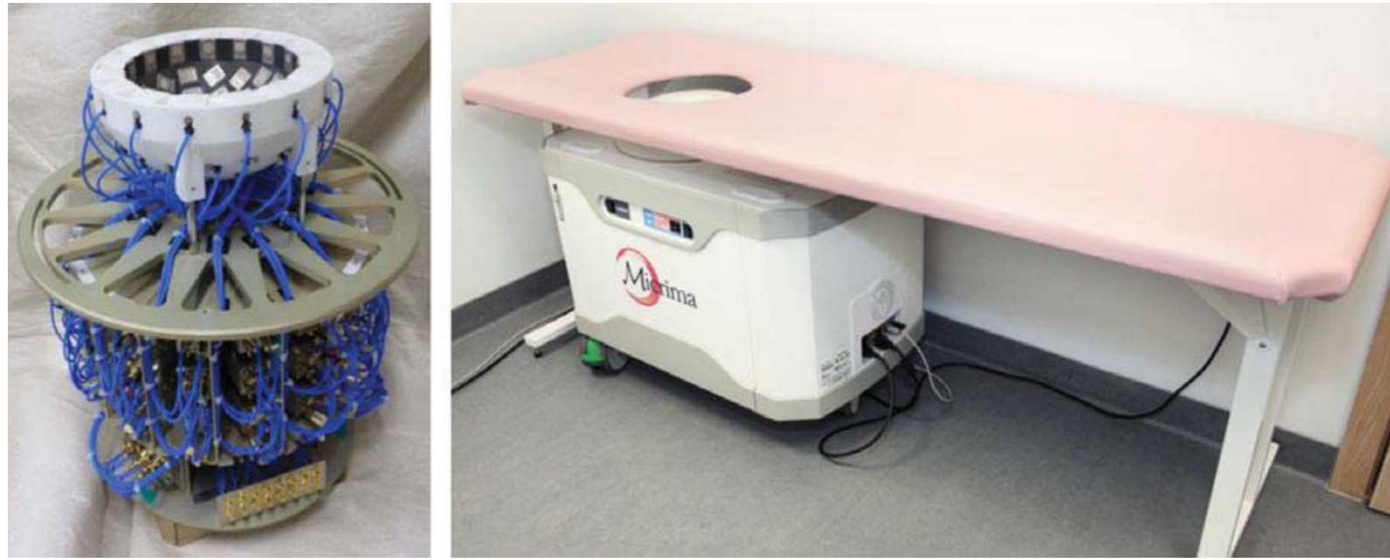
Radar-based microwave imaging system (Bristol University, UK)
