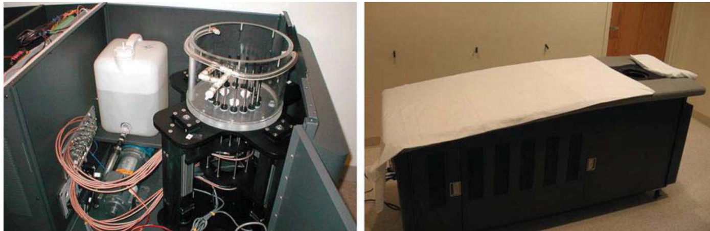
3D tomography microwave imaging system (Dartmouth University, USA)
