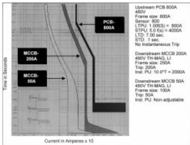
Fig. 3. Time-current curve with upstream 800-A PCB.
