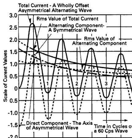
Fig. 1. Structure of an asymmetrical current wave.
