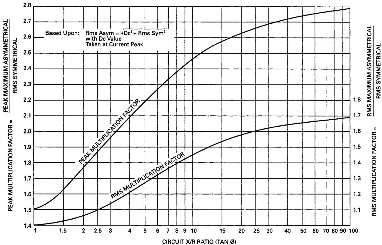
Fig. 2. Relation of  $X/R$  ratio to multiplication factor[15].
