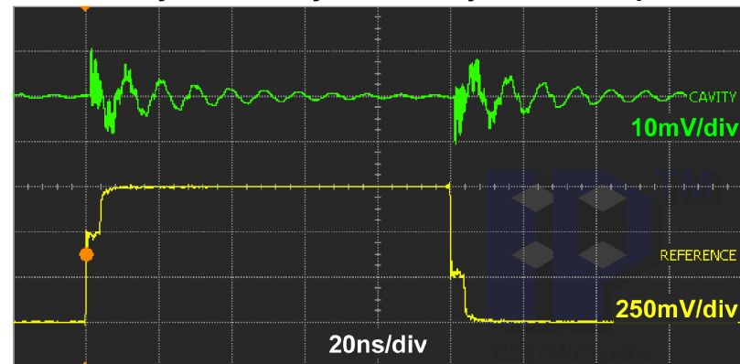
Cavity Disturbance Single 0 Ohm Resistor Plane to Plane 2" Layer 1 -> 2" Layer 4 -> 2" Layer 1 Microstrip
