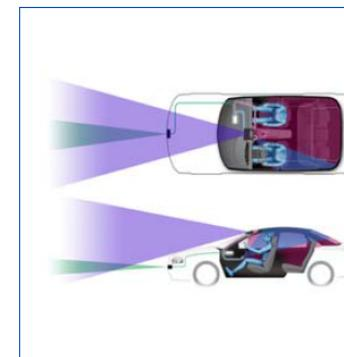
Data fusion algorithms combine inputs from radar and vision sensors to enhance safety system functionality.
