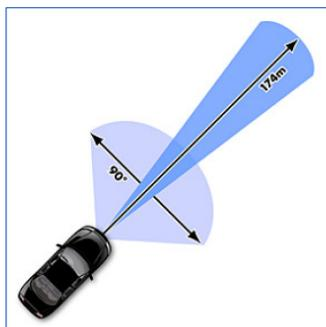
Wide mid-range coverage not only allows vehicles cutting in from adjacent lanes to be detected but also identifies vehicles and pedestrians. Long-range coverage provides accurate range and speed data with effective object discrimination.
