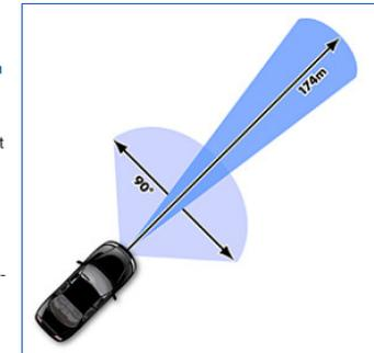
Wide mid-range coverage not only allows vehicles cutting in from adjacent lanes to be detected but also identifies vehicles and pedestrians. Long-range coverage provides accurate range and speed data with effective object discrimination.
