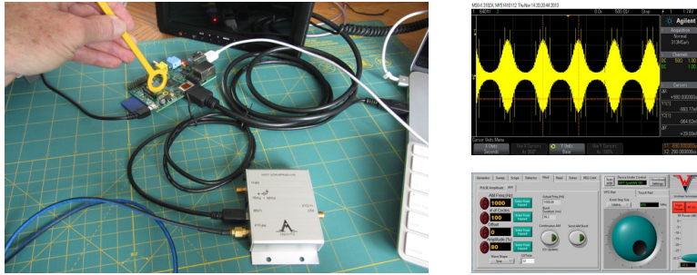
Using the Windfreak Technologies "SynthNV" RF synthesizer with 80% AM modulation to test radiated immunity.
