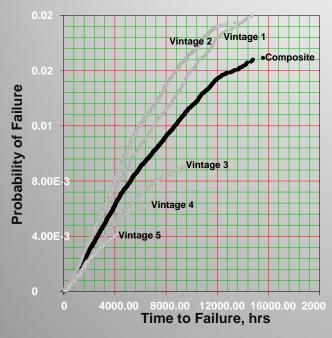
Slightly decreasing failure rates, then increasing rate (esp. HDD#2)
