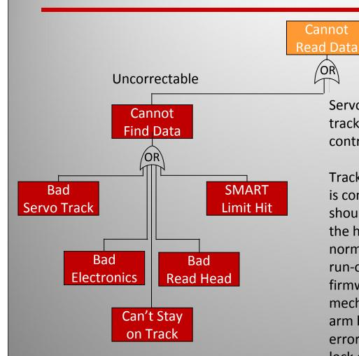
Servo data is written at regular intervals on every data track of every disk surface. The servo data is used to control the positioning of the read/write heads.
