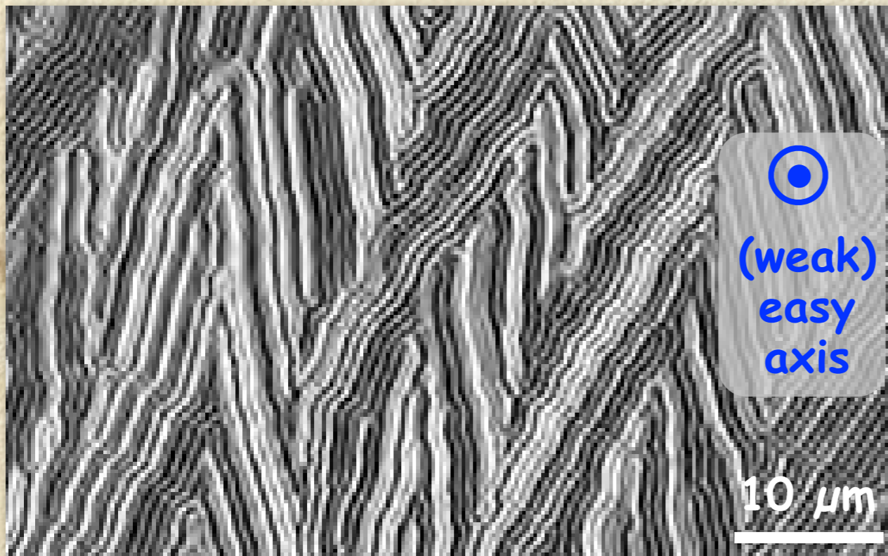
Amorphous FeSiBCuNb film, 2 \mu\text{m} thick
