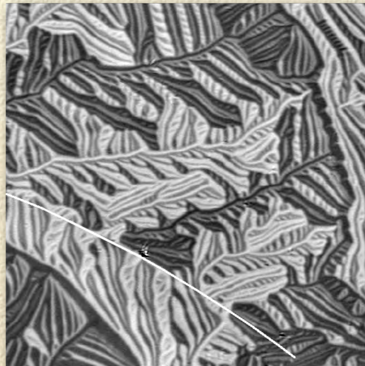
Branched closure domains in medium-Q bulk material
