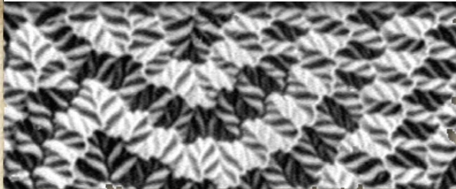
Branched closure domains in low-Q bulk material
