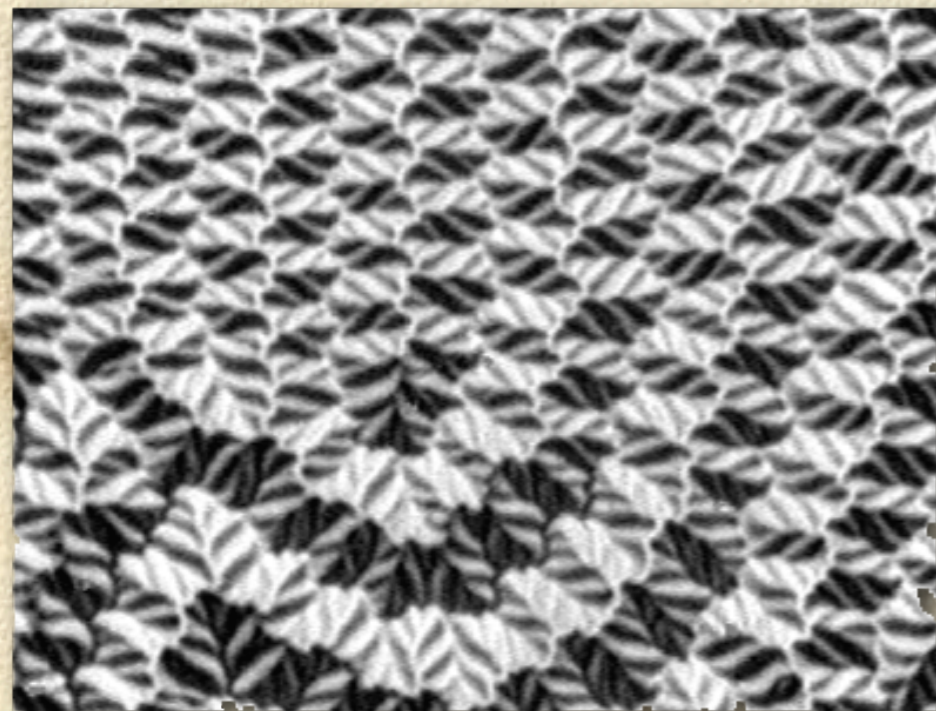
Branched closure domains in low-Q bulk material
