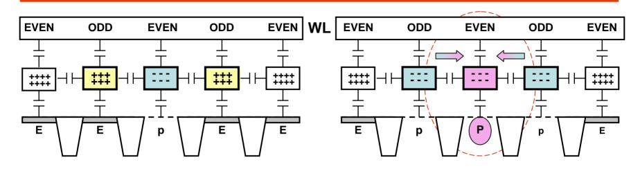
Additional negative voltage in a two-step sequence for Floating Gates programmed in step TWO (Yupin Effect\*)
