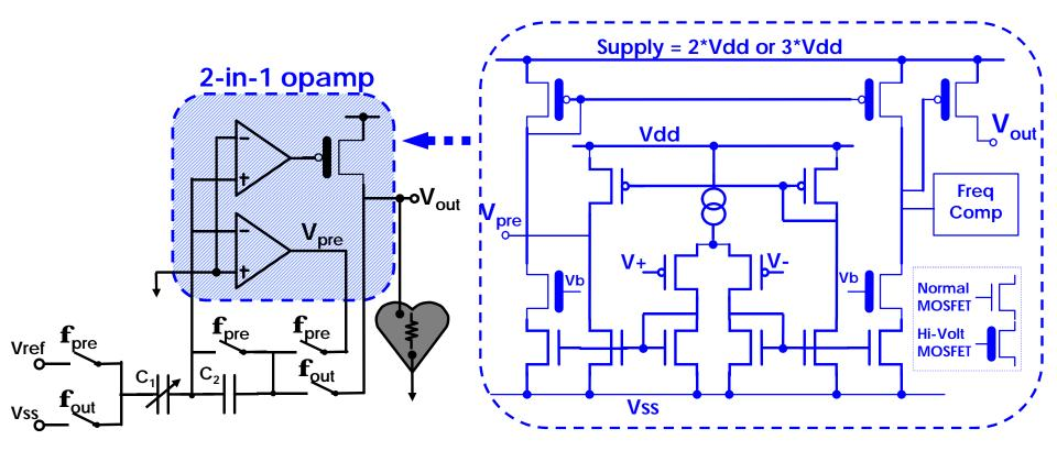
High-Voltage DAC utilizing 2-in-1 opamp 2-in-1 (HV/LV) CMOS opamp
