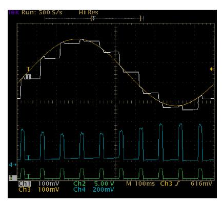
SHA with Leakage Cancellation 1Hz sine input, Fs=10Hz I leakage < 0.01pA (effective)
