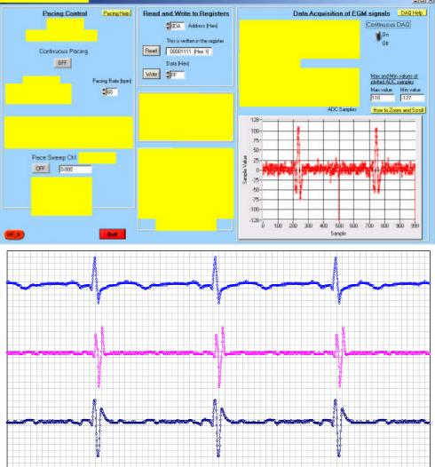
An example ADC output of Electrocardiogram (ECG) processed by different SC filters.
