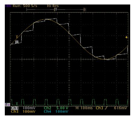
SHA (Original) 1Hz sine input, Fs=10Hz I leakage ~ 0.1pA total
