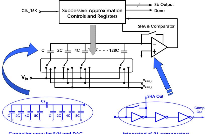
Capacitor array for S/H and DAC
