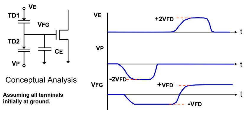
Voltage swing on FG conceptually 2VFD ( = 24V for 12V VFD) Large VFD voltage improves dynamic range and signal-to-noise ratio
