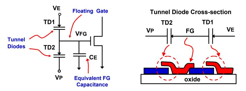
FG is isolated by oxide and cannot gain or lose charge under normal conditions
