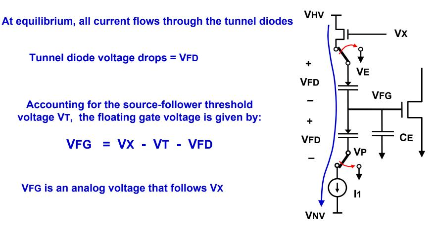
When both switches are connected to ground, charge is trapped on the floating gate and now VFG is a stable D.C. voltage
