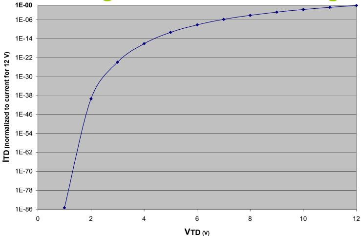
The TD current drops 38 orders of magnitude from 12V to 2V →Loss of 1 electron in several Trillion years @2V →16nV drift for a 10pf Storage capacitor
