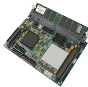
Fig. 1a: ARM RealView ® Validation System Board
