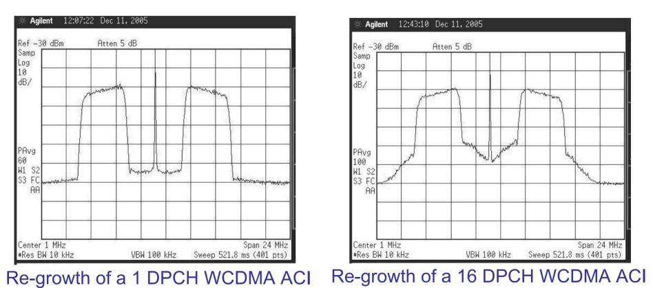
High PAR/increase in channels in adjacent channel will cause increased spectral re-growth.
