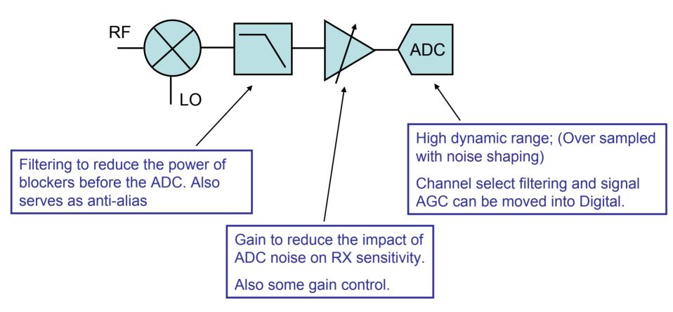
• High dynamic range in the ADC reduces the filtering and gain required in the analog (lower analog signal processing).
