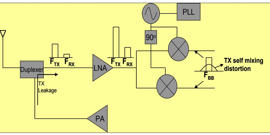
Figure showing IM2 distortion from modulated TX blocker in FDD mode.
