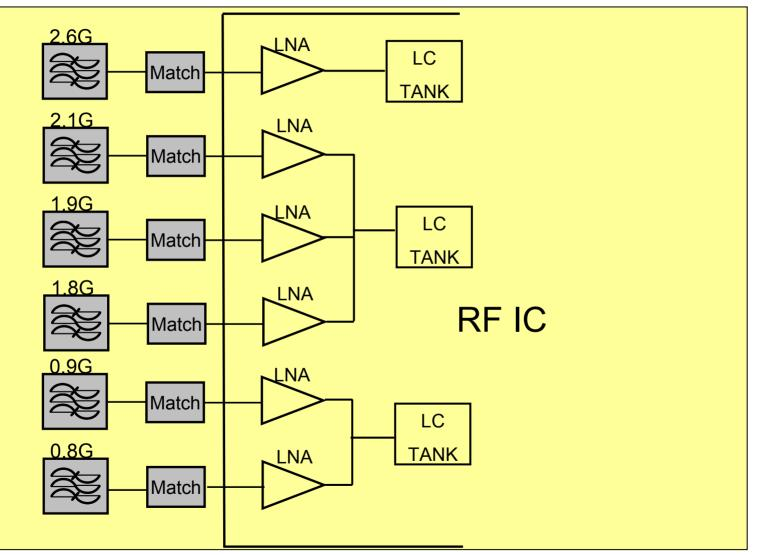
> Dedicated RX input pins, Matching Networks, LNA input stages are required.
