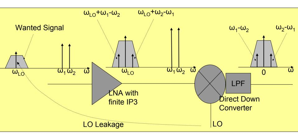
$\omega_1 - \omega_2, \omega_2 - \omega_1$  at the output of the mixer looks like an IM2 component. (Can misleadingly imply an IP2 issue!)
