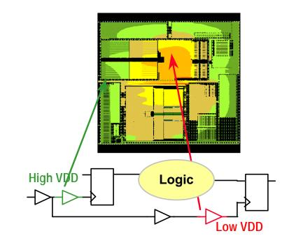
Delta VDD  $\rightarrow$  Hold time failure
