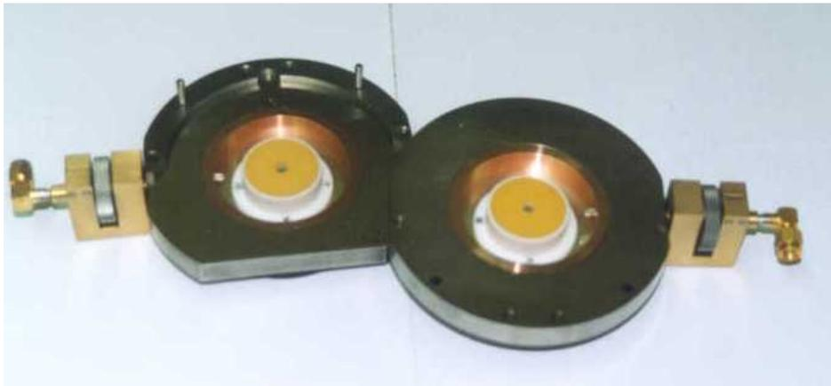
Dissassembled 3.2 GHz split post
