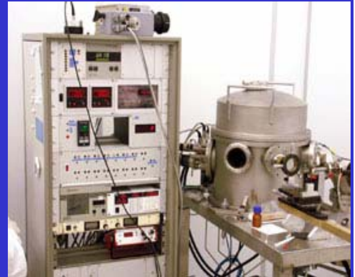
PLD System - MC2 Process Lab Chalmers
