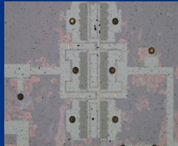
80 \mu\text{m} diameter through wafer via-holes on an MMIC chip
