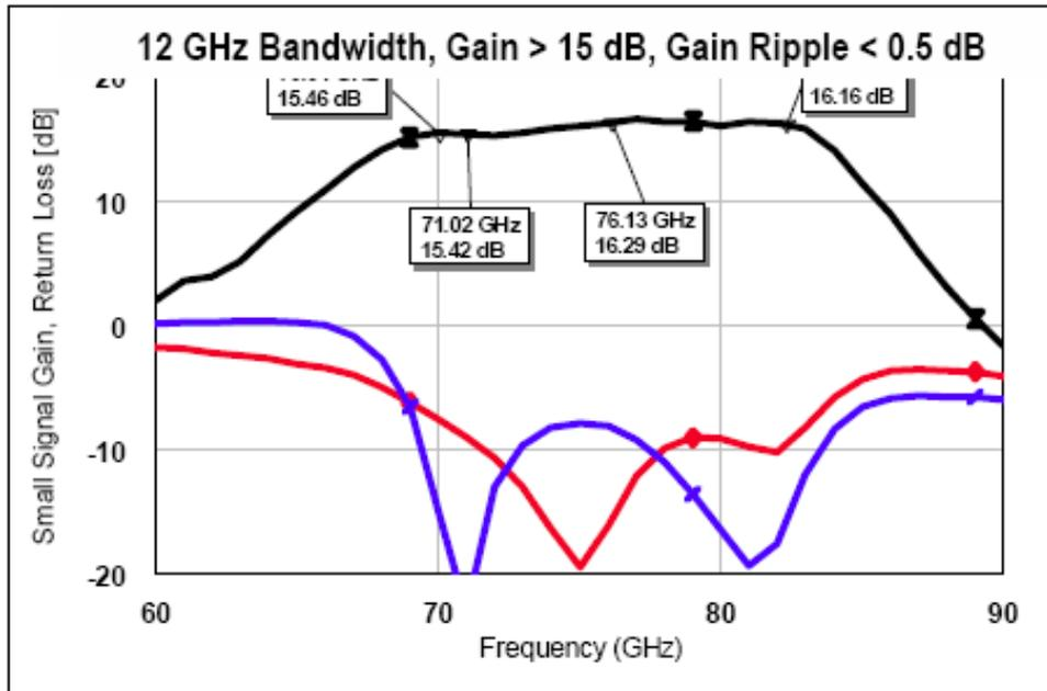
Measured small signal gain of 70 GHz 500 mW GaN MMIC PA.
