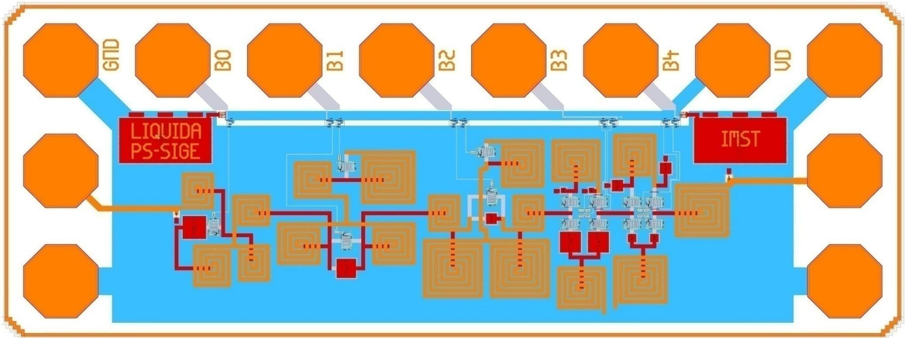
$V_D = 3 \text{ V}$ ,  $V_C (B0-B4) = 0 \text{ V} / 3 \text{ V}$  (active / not active)
