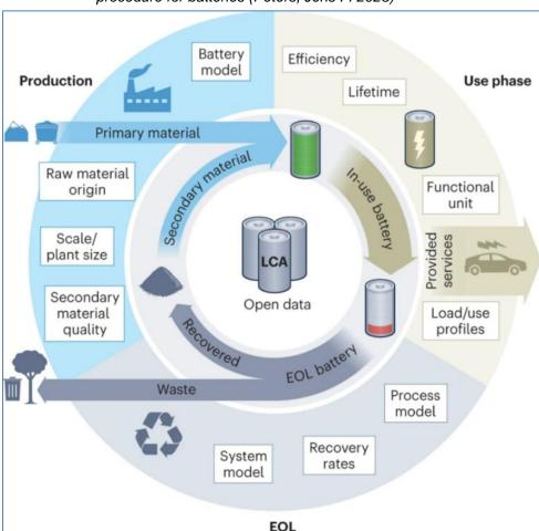
Figure: Schematic representation of the assessment procedure for batteries (Peters, Jens F. 2023)
