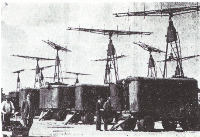
TRUCK-TRAILER units, with the spidery antennae whirling like Dutch windmills, send out the radar signals. They move in four pieces—two trucks and two trailers. The exacting work of assembling the intricate mechanisms of radar units was one of the jobs assigned to Canadian war plants. One was Research Enterprises Ltd., Leaside.
