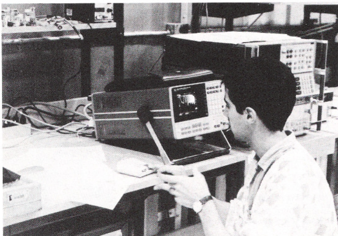
Test Technologist Morris Scarpino measures low frequency radiated magnetic fields with the product under test in the RF anechoic chamber. The test is being conducted to MIL-STD-462, RE01.
