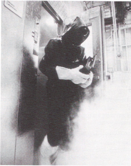
Test Technologist Duane Friesen exits the walk-in chamber after performing a functional test on a commercial product which is undergoing a -55^{\circ}\text{C} low temperature test.
