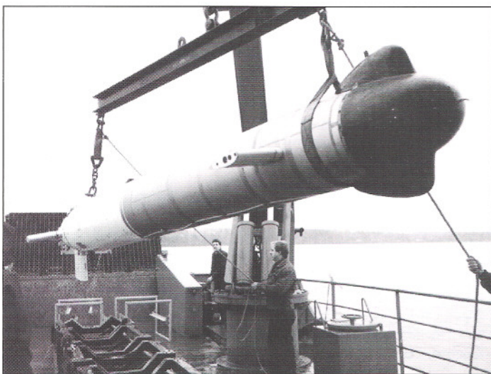
Figure 3. ISE ARCs Autonomous Underwater Vehicle being launched from the ISE boat "Researcher". Typical applications include under-ice hydrographic survey and oceanographic sensing. (ISE)
