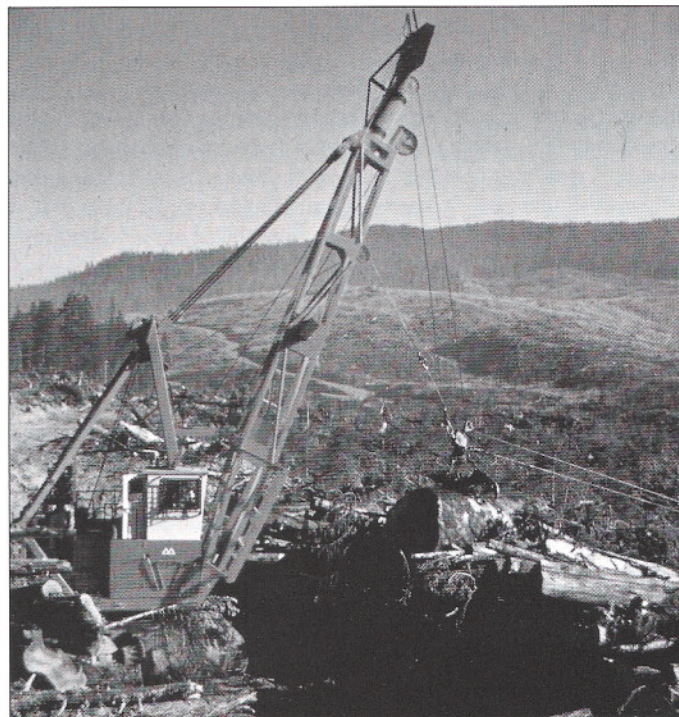
Figure 1 : The Madili grapple yarder operating in Coastal British Columbia
