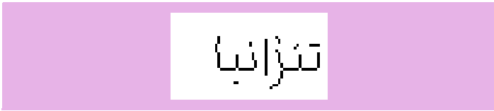
Figure 2: The Word 'Tanzania' in Arabic, after the application of a Thinning Algorithm [8]
