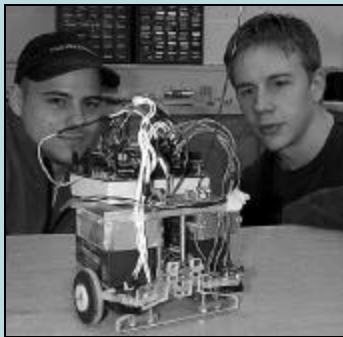
Figure 2: Students Victor Haramina (left), Brian Johnson (right) are shown with their soccer playing robot. Ron Tezuka was also part of the group. This group was one of two groups which designed a kicking device. This group used a solenoid for the kicking device which required a larger battery back.
